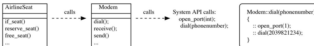
Figure 18.3: Indirect coupling to an unstable interface.
